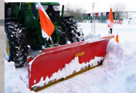
Snow blade, material thickness 5-6 mm steel plate
