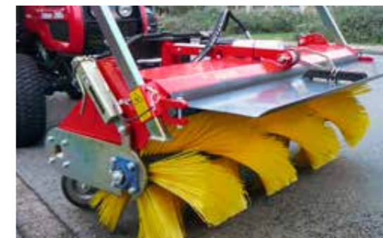
K 560 with adjustable splash guard
