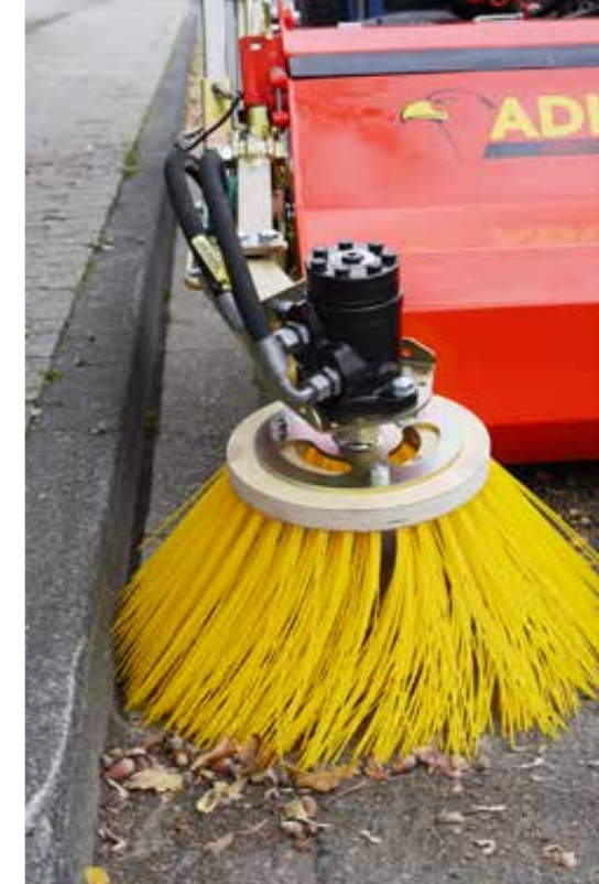
Rotary side brush in use
