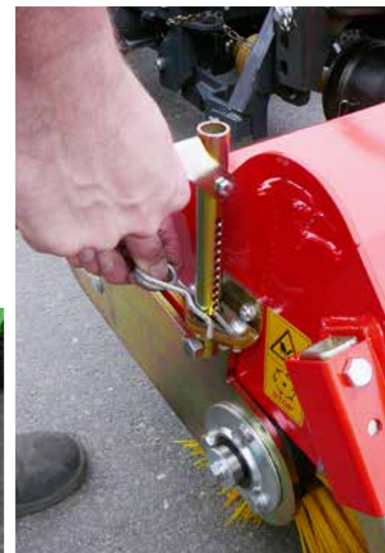
Brush adjustment via push-fit system
