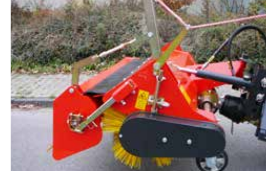
K 450 with mechanical hopper emptying
