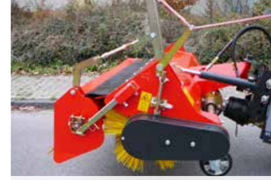
K 450 with mechanical hopper emptying
