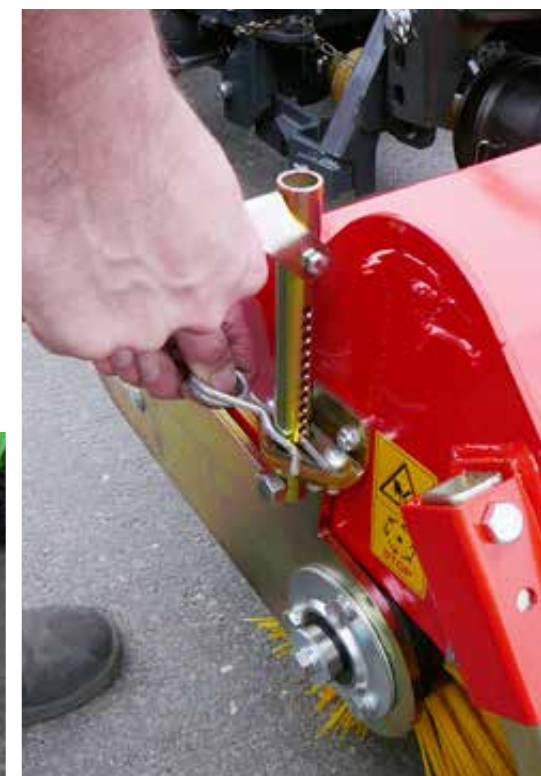
Brush adjustment via push-fit system
