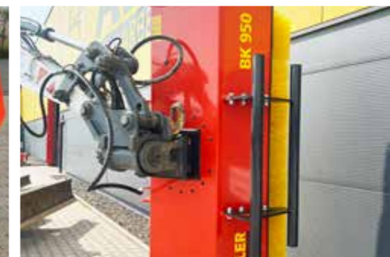
Insert for vertical use with power tilt function on the backhoe
