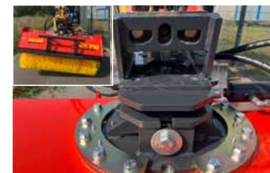
Spring-loaded pendulum adapts perfectly to the ground
