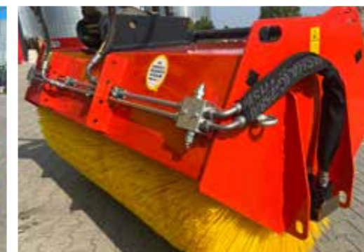
Powerful hydraulic motors with motor-preserving overrun protection
