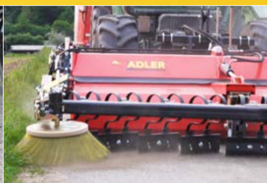
With ADLER everything goes well: sweeping machine with dirt collector, scraper and side brush
