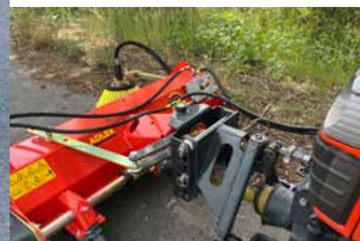
Hitch system hitch triangle Kat. Municipal
