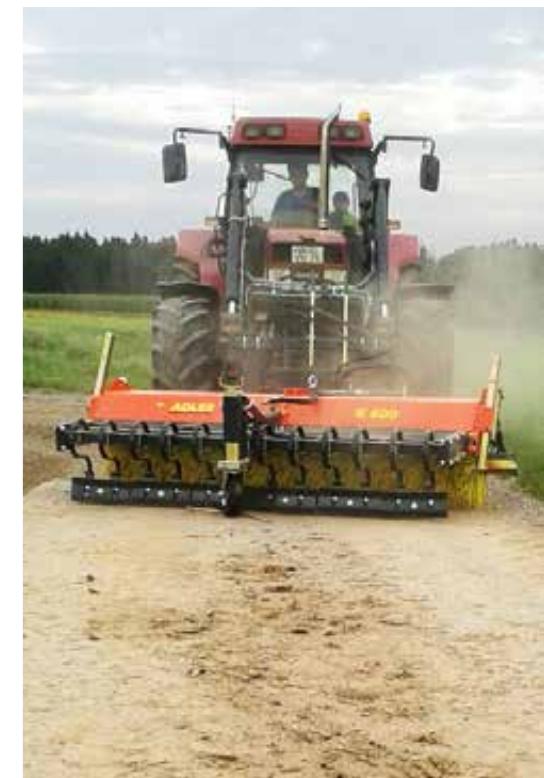
KV-series Scraper attachment with third support wheel
