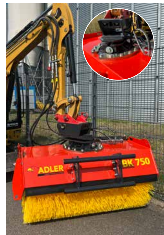
Slewing ring to turn the machine 90° – hydraulically or mechanically
