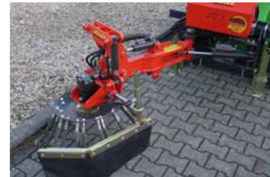
Heavy brush head with protective side guard
