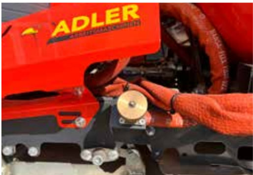
Side fill inlet for LPG autogas
