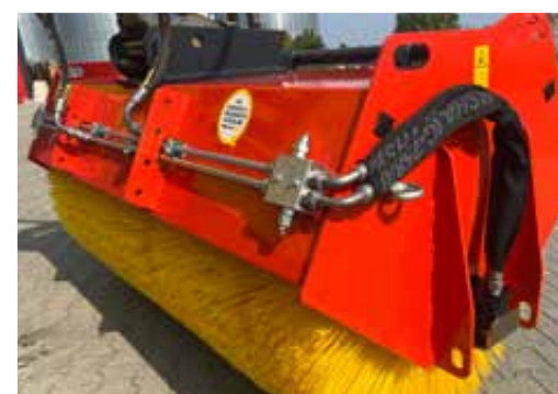
Powerful hydraulic motors with motor-preserving overrun protection
