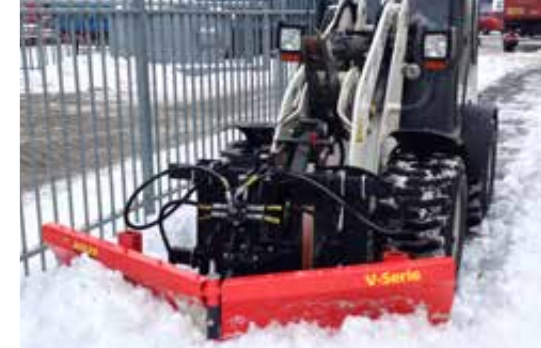
V-series attached to yard loader
