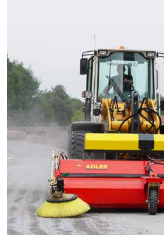
Side brush and water spray systems as an option
