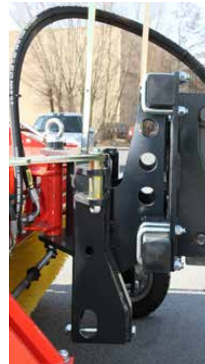
Wheel loader hitch with roller guide system and 3D leveling
