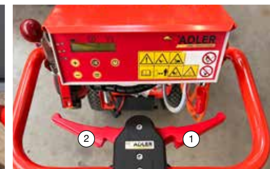
Driving lever for 1) forward and 2) backwards
