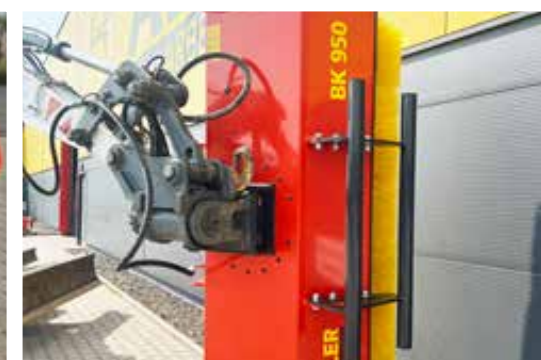
Insert for vertical use with power tilt function on the excavator
