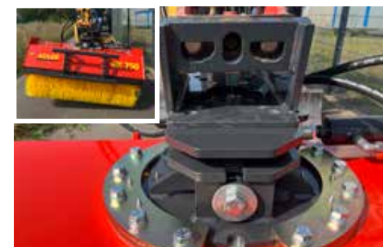
Spring-loaded pendulum adapts perfectly to the ground
