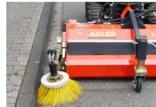
Rotary side brush in use with support wheel
