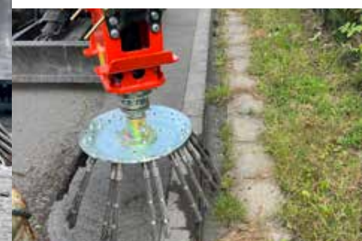
Right/left rotation as standard for individual cleaning scenarios
