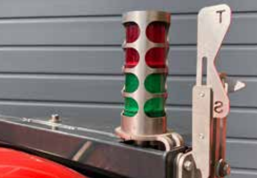
Indicator for height adjustment and signal lamps for infra box operating control
