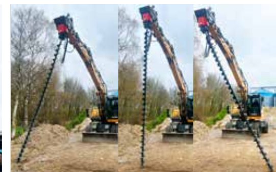
Simple handling – thanks to the integrated 2D pendulum travel
