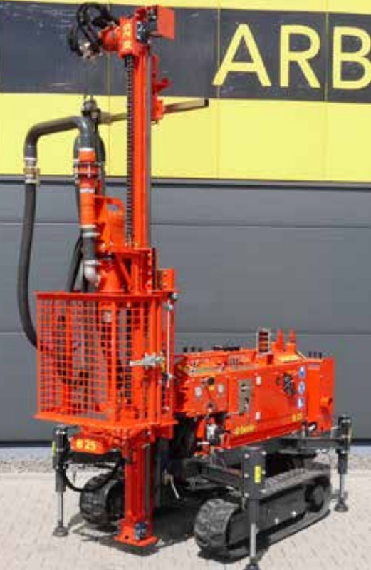
ADLER-Drill Rig on ADLER-Crawler Undercarriage
