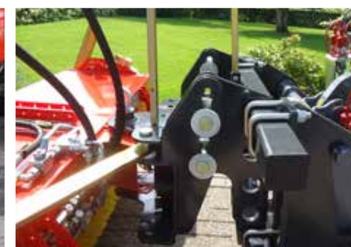
Universal attachment with 3D leveling system
