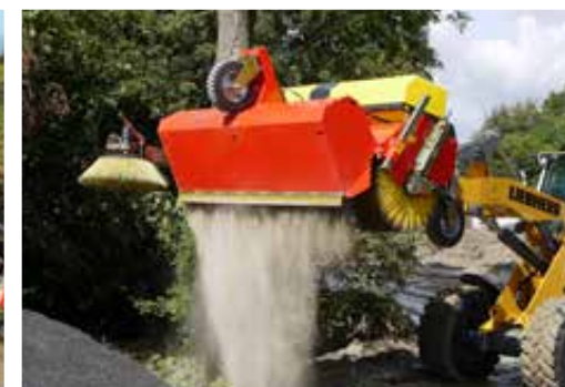
Hydraulic hopper emptying system
