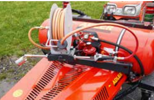
Available on option: Hand-held burner kit incl. 15 m-hose reel
