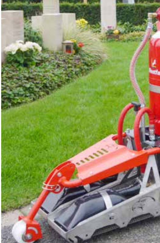
The front wheel ensures that the infrared emitter is positioned at the optimum working height
