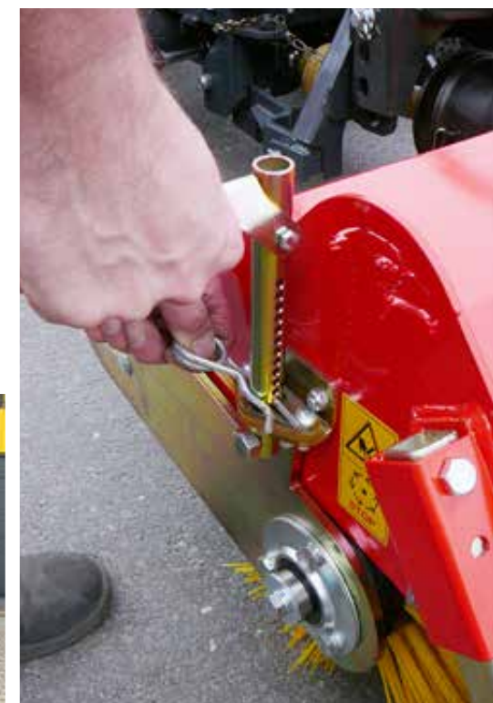
Brush adjustment via push-fit system
