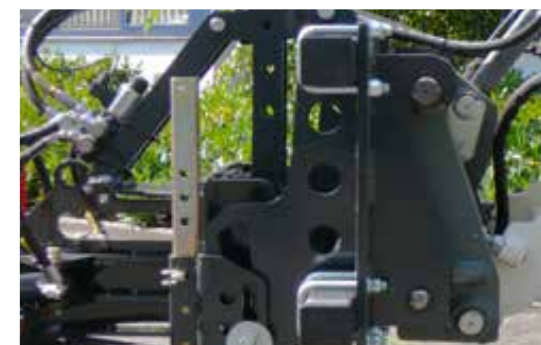
Universal attachment with leveling system and parking stand
