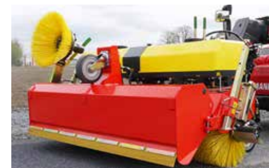
Simple sweeping mode, hydraulic hopper emptying system and 3rd support wheel on hopper
