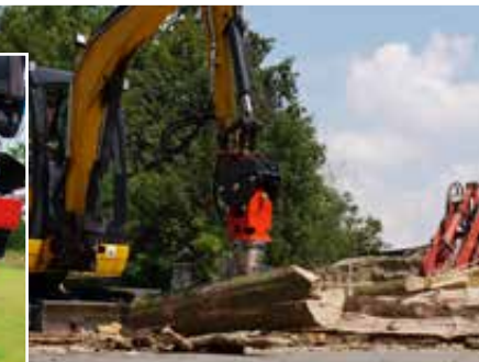
Splitting and stacking in a single work process
