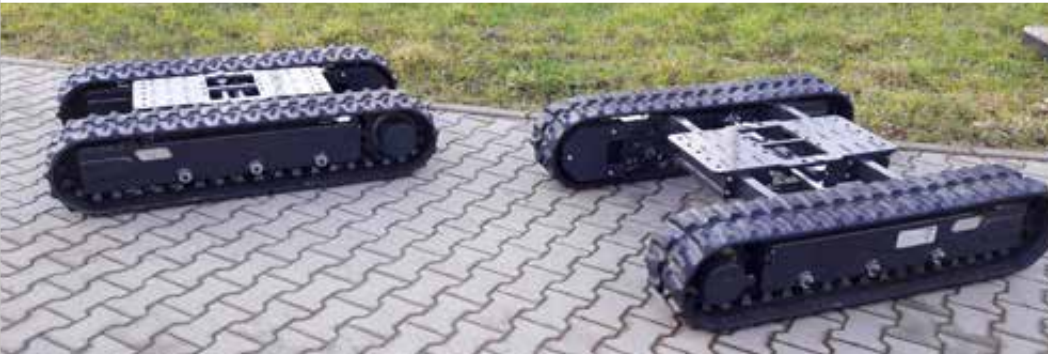
The undercarriages can be manufactured either hydraulically telescopable or without a center section
