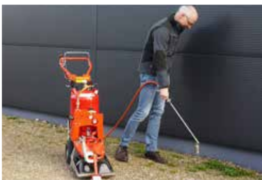
The hand-held burner allows treatment of even difficult-to-access terrain
