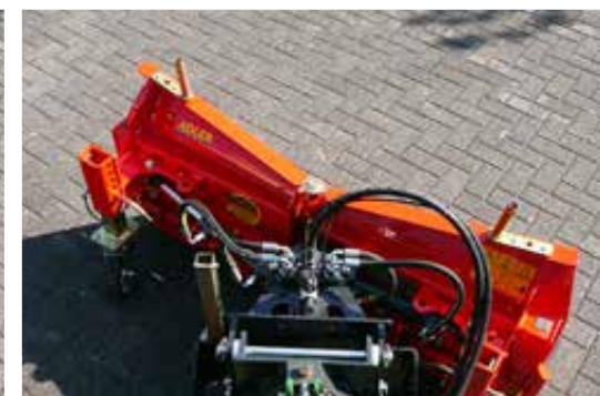
Universal attachment with leveling system and parking stand
