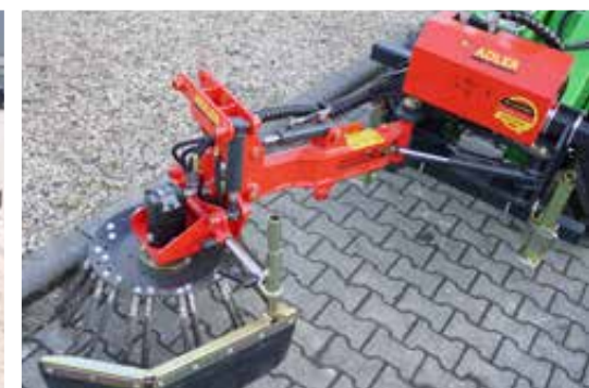
Hydraulically adjustable grade and transverse slope, on option also mechanical adjustment possible
