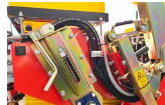
Brushes are continuously adjustable
