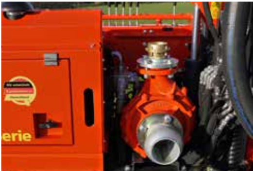
Spülpumpe "on board"
