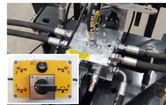
Electric switch valve with overload protection provided by two pressure relief valves and nitrogen bubble
