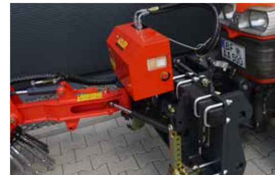
Universal attachment with lateral pivoting
