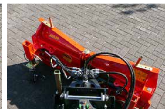
Yard loader with levelling system and parking stand
