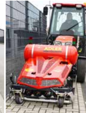
Hydraulic side shift 20 cm to the left and right
