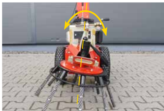
Stepless adjustment of handlebar height
