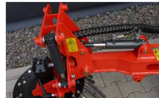
Hydraulically adjustable grade and transverse slope, on option also mechanical adjustment possible
