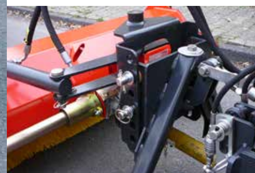
Hitch system hitch triangle Kat. Municipal
