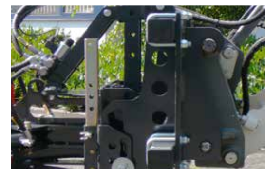
Yard loader with levelling system and parking stand
