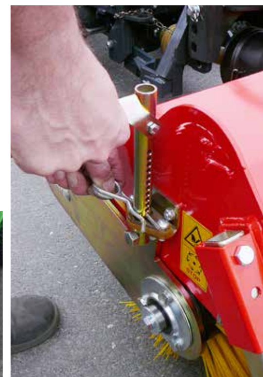
Brush adjustment via push-fit system
