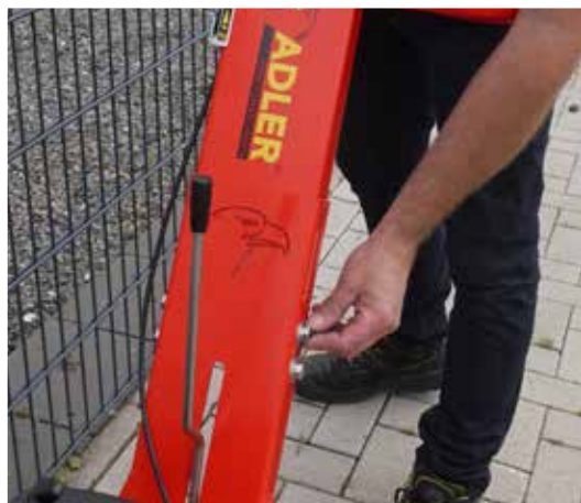
Stepless adjustment of handlebar height
