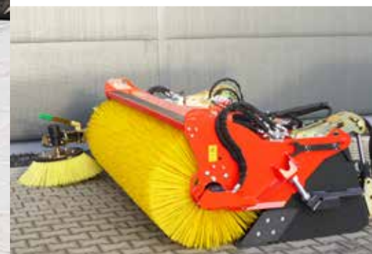
Sweeping bucket optionally available with rotary side brush
