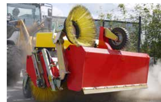
Simple sweeping mode and 750 mm brush diameter as standard features
