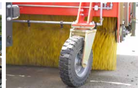
Three large wheels 400 mm x 100 mm
