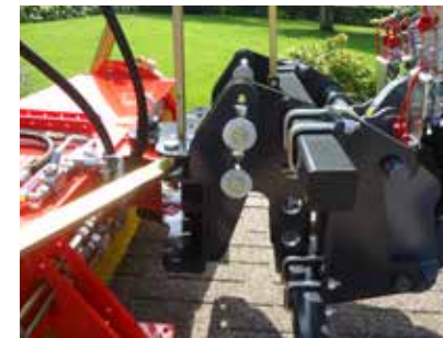
Wheel loader hitch with roller guide system and 3D levelling
