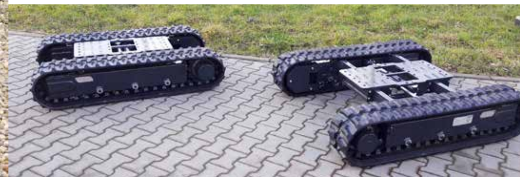
All undercarriages can be manufactured in a rigid version or with hydraulic telescoping.
