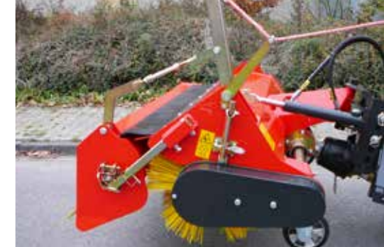
K 450 with mechanical hopper emptying
