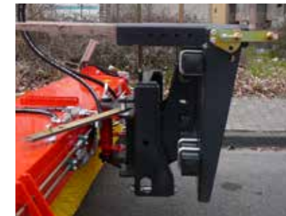
Combined wheel loader/fork lift attachment incl. roller guide system and 3D levelling
