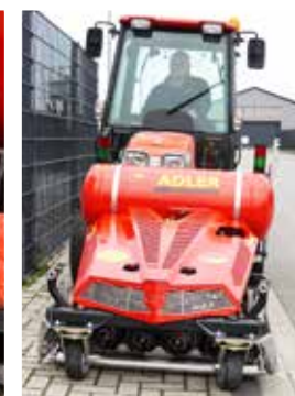
Hydraulic side shift 20 cm to the left and right
