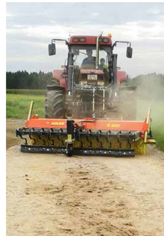
KV-series Scraper Attachment with third support wheel
