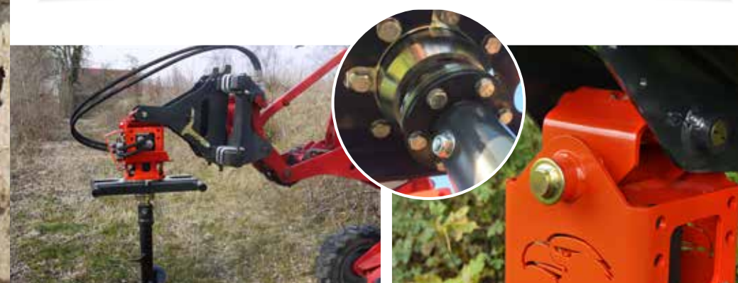
Universal joint and front bearings featured as standard
