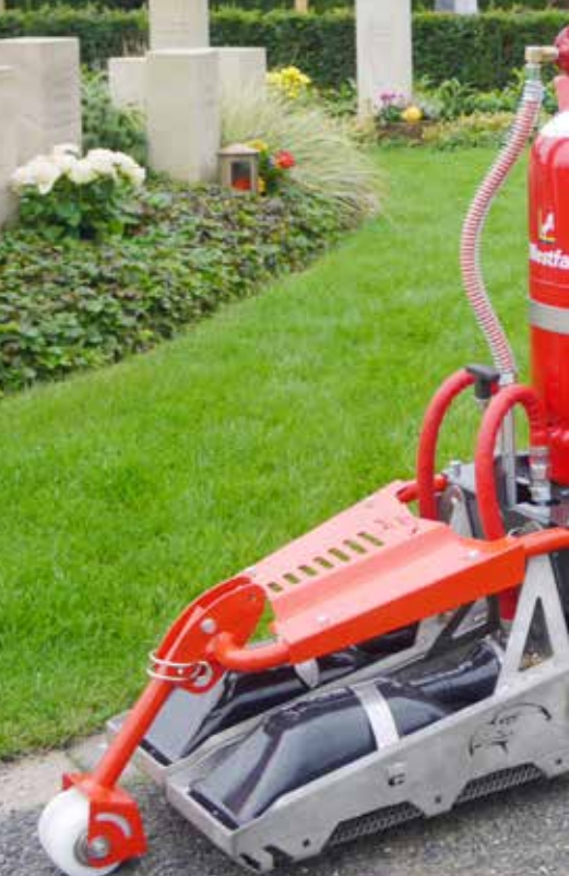
The front wheel ensures that the infrared emitter is positioned at the optimum working height.
