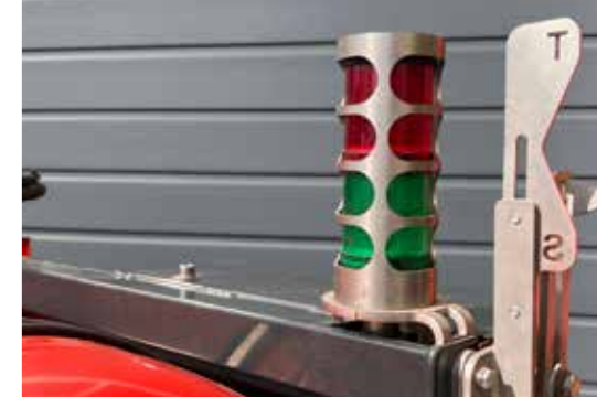
Indicator for height adjustment and signal lamps for infra box operating control
