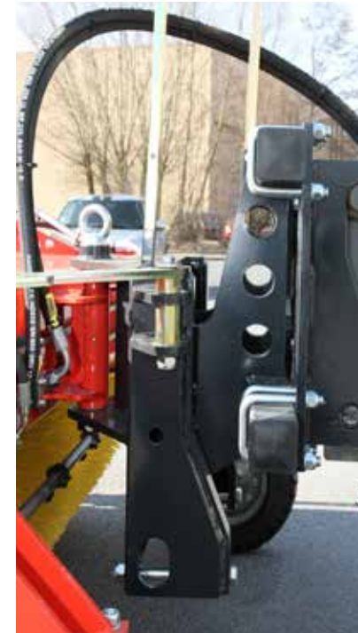
Wheel loader hitch with roller guide system and 3D levelling
