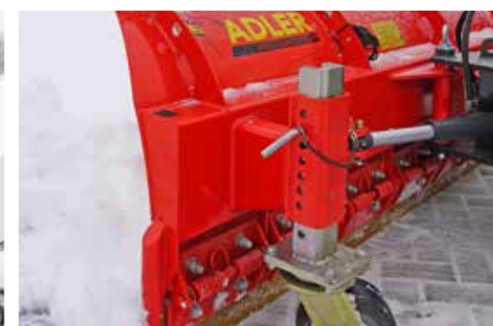
Height-adjustable support wheels (200 x 80 mm)
