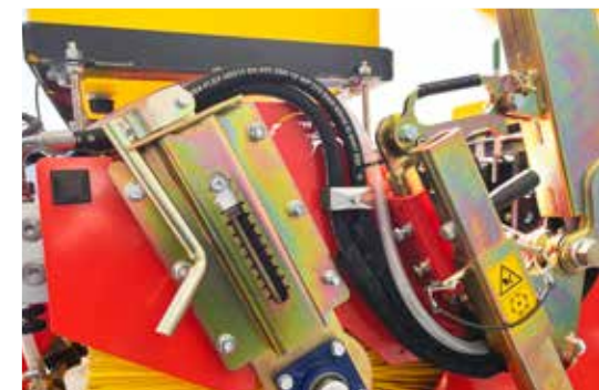
Brushes are continuously adjustable
