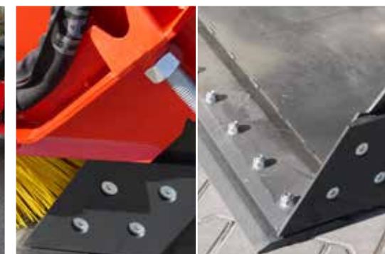
Interchangeable wear-resistant cutter
