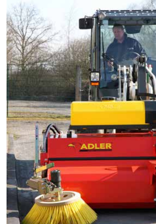
Optional rotary side brush and 240-l water tank
