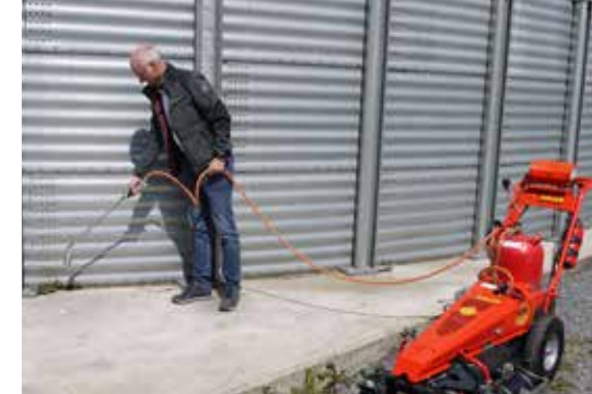
Hand-held burner for difficult-to-reach corners and edges
