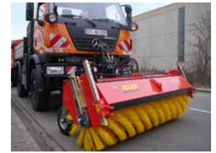
Unimog Attachment incl. lifting system acc. to DIN 76060
