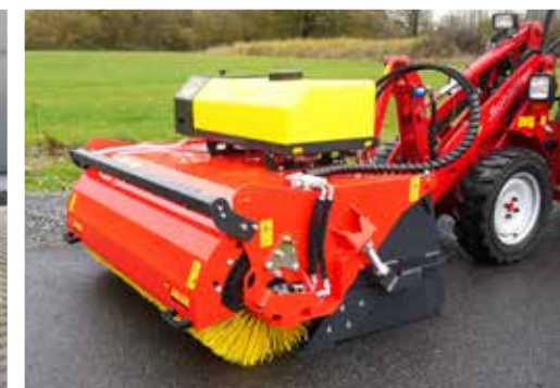
KS 600 mounted on a wheel loader incl. water-spray system
