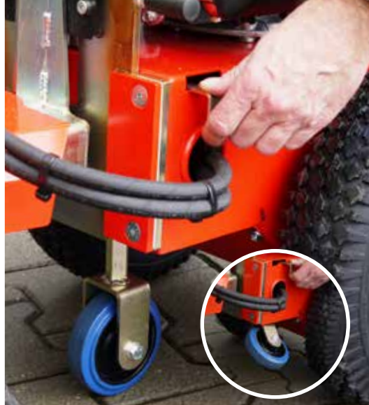
Depending on the area of application the support wheel can be comfortably folded in and out.
