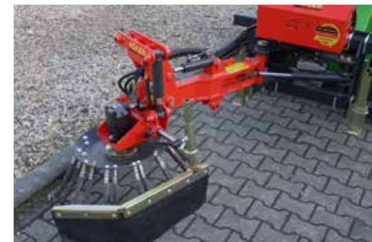
Heavy brush head with protective side guard
