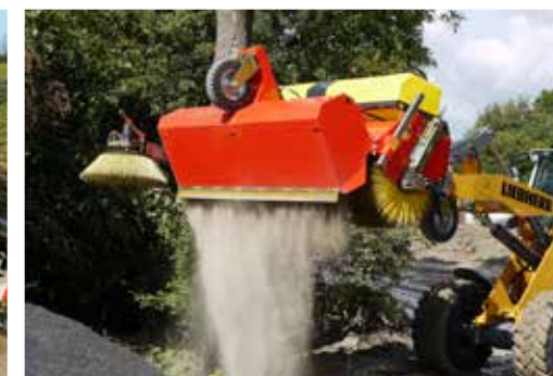
Hydraulic hopper emptying system
