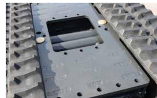
The centre piece of the undercarriage has many fixing points for customer-specific use.
