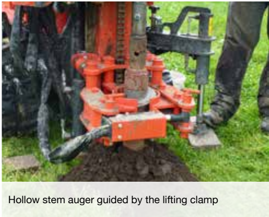
Easy disassembly of the hollow stem auger due to the swivel-out drill head
