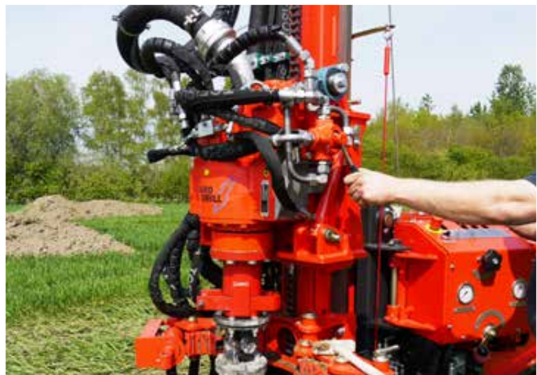
2-stage drill drive with torques up to 620 daNm or revolutions up to 210 rpm
