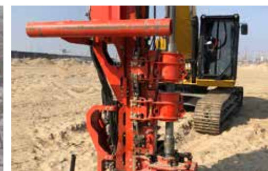
Cable-crushing-lifting clamp in use
