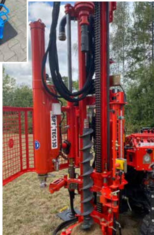
Geological probing with the pile-driving probing unit or the hollow stem auger possible in alternation
