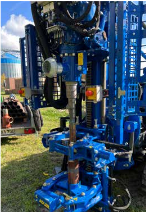
Cable-crushing-lifting clamp in use
