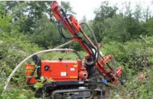
B 25 with offset drilling attachment
