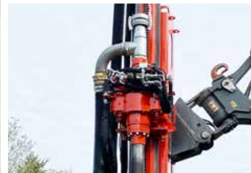
Attachment drill mast with hydraulic clamp
