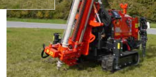
15° mast tilt to the right / left / front
