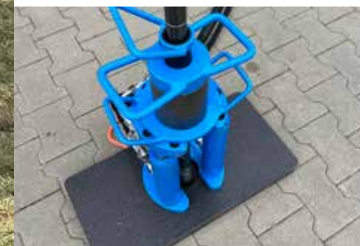
Lifting unit with ball clamp for pulling the pile-driving or pile-coring tools (120 kN lifting force)
