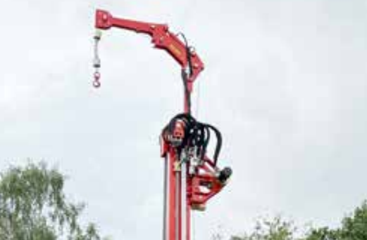
Winch with cable stopper and mast extension
