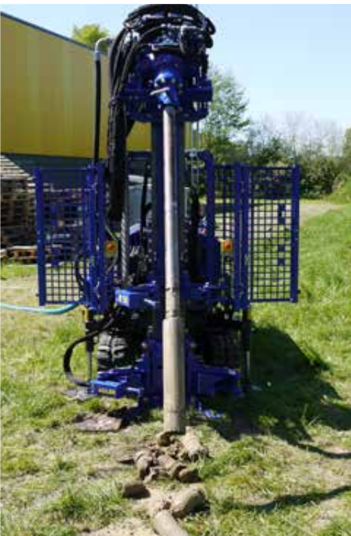
Core drilling with single core drill pipe or double core drill pipe
