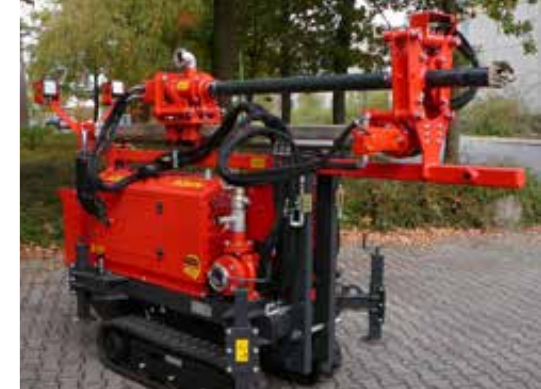
B 15 the compact drill rig for shallow depths
