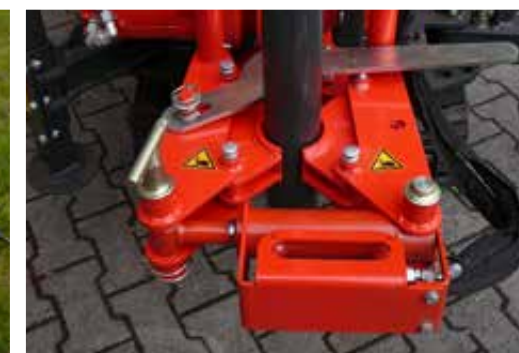
Hydraulic drill pipe breaker
