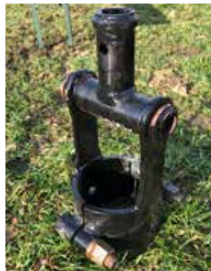
Removal clamp for the outside piping
