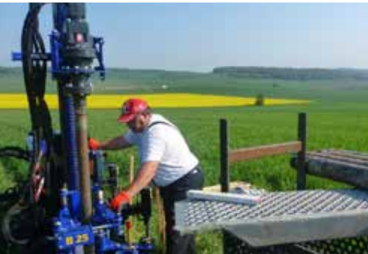
B 25 drill rig in use pulling cores
