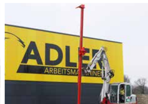
Attachment drill mast with hydraulic clamp
