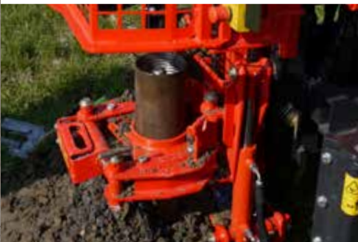
Optional for B 25: Lifting clamp for drilling cased boreholes
