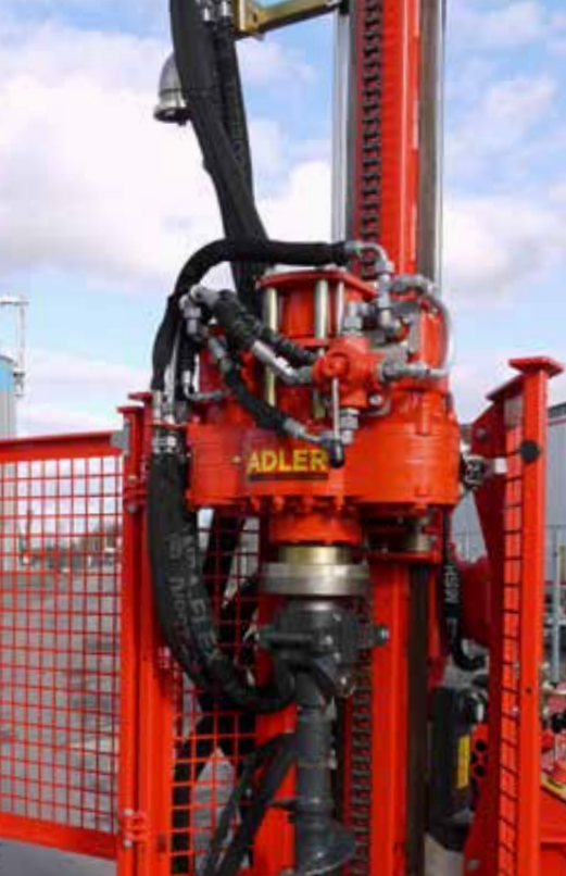
Geared drill head with two switching stages
