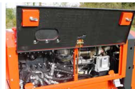
Drill rig B 75 equipped with 75 HP and 2.9 litre Deutz engine of the latest emission standard 5
