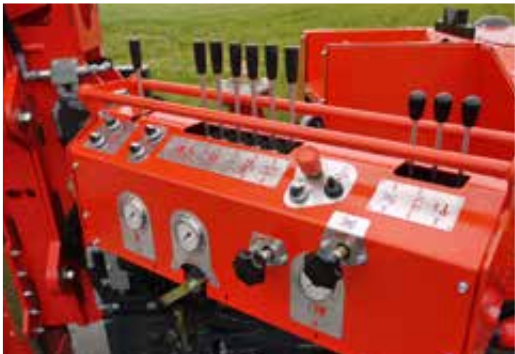
Fold-out control panel for the control of all important drilling functions
