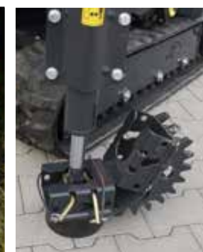
Support shoe set for grass and indoor use with anti-slip system
