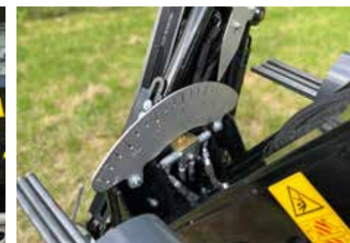
Angular measuring unit for oblique hammering
