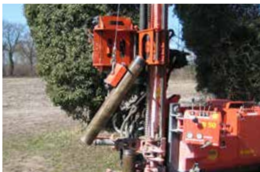
A magnetic winch supplies drilling accessories during the drilling process
