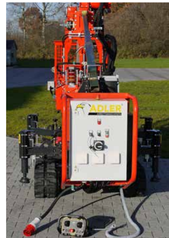
Electric control cabinet with three CEE sockets (outlet)
