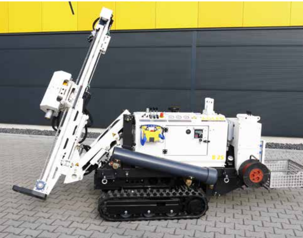
3D-ram drill rig with hydraulic hammer
