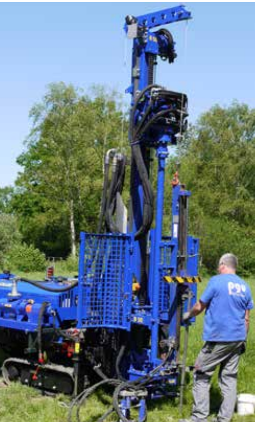
Dynamic probing with the ADLER-drill rig B 50
