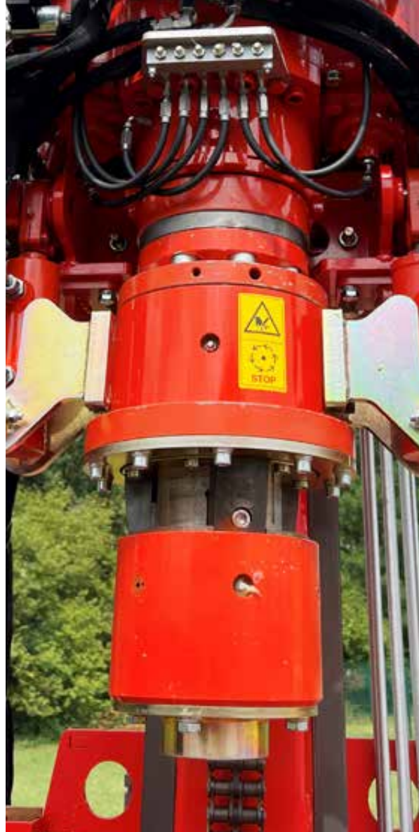
Hydraulic clamping bell (large/small) for breaking the drill pipes and the outer pipework up to 178 mm (only possible with large clamping bell)
