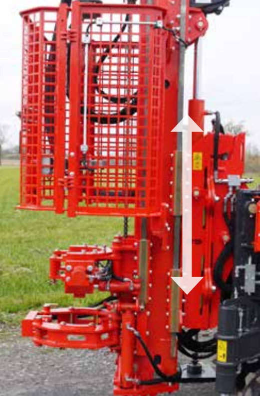
Mast lowering by 300 mm at B 75 per standard
