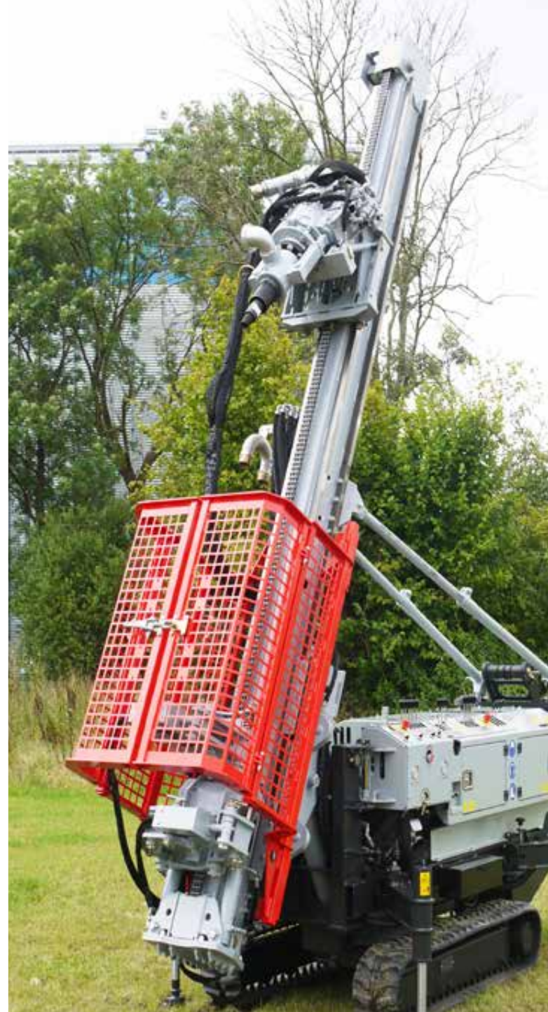
Oblique drilling device with mast supports
