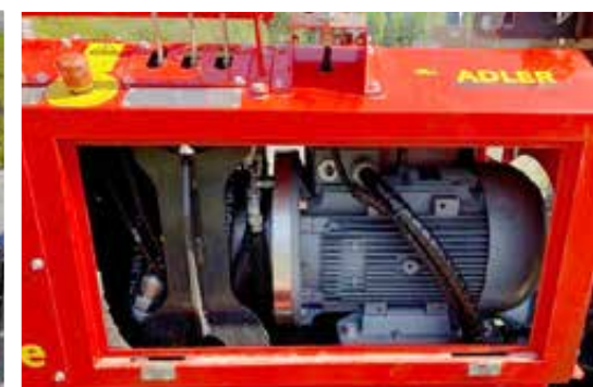
Emission-friendly electric motor 18.5 kW - 380 V - 3,000 rpm
