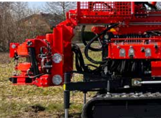
Piping turntable in transport position
