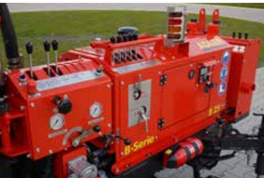
Operating station with all drill functions – pivot mechanism
