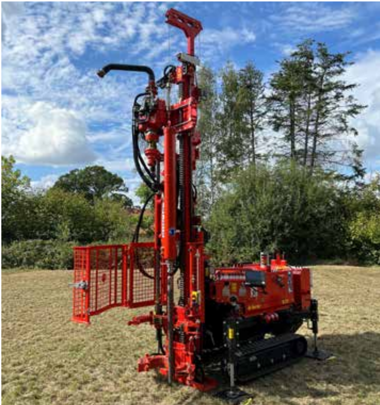
B 25 equipped with a percussion probing unit
