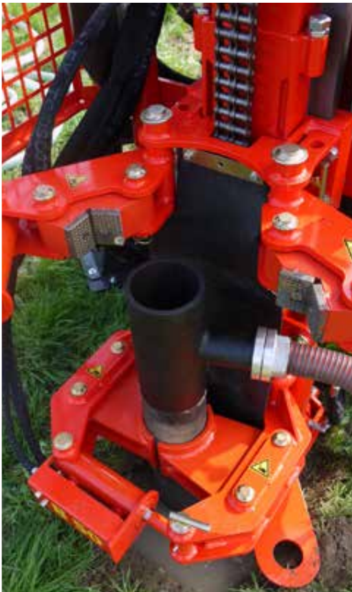
Water drainage during core drilling
