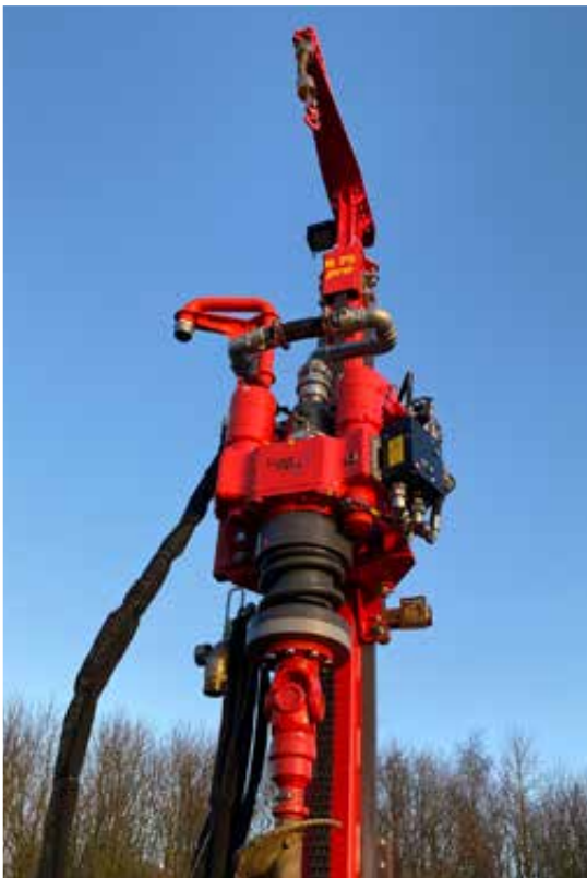
Gear drill head with floating spindle on B 75 pro
