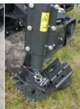
Support shoe set for grass and indoor use with anti-slip system
