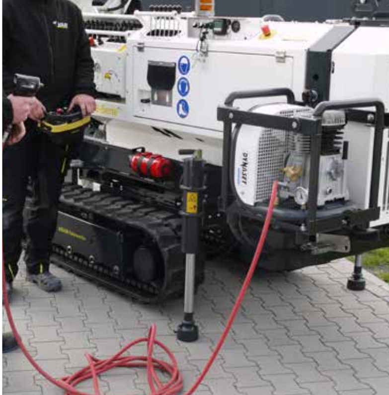
Air compressor – drive via the drill rig
