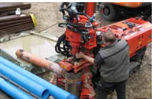
Breaker with hydraulic clamp – standard feature on all B-series models
