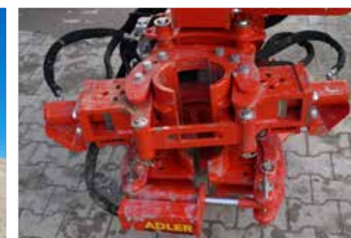
Mast foot designed as a cable-crushing-lifting clamp
