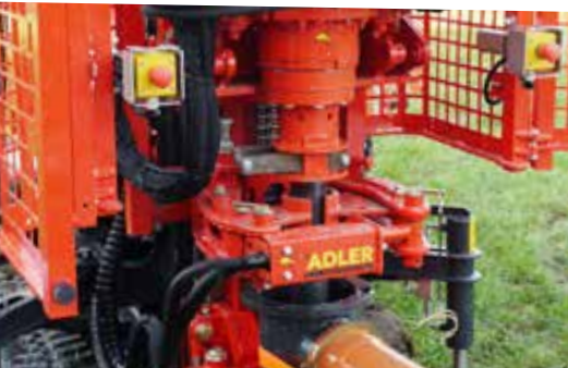
Lift clamp and hydraulic drill rod breaking bracket
