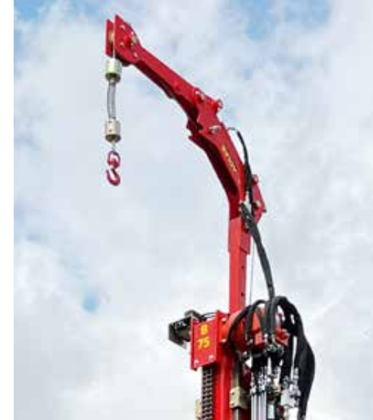
Winch with cable stopper and mast extension
