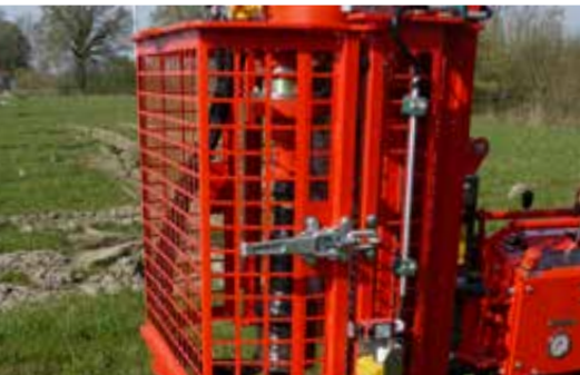
Safety device around rotating pipe fitted as standard
