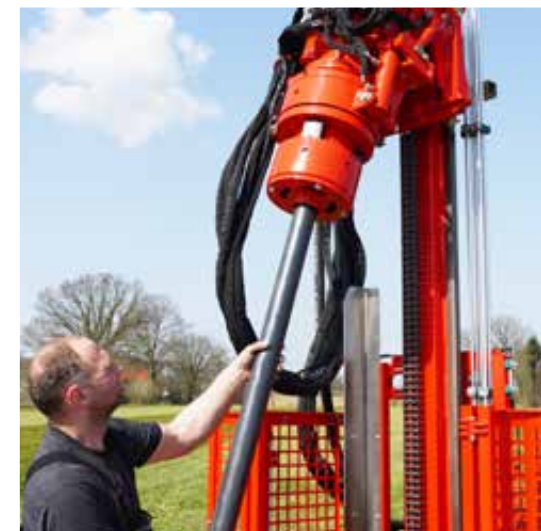
Hydraulic clamping bell (large) to the drill pipe and to break the outer piping up to 178 mm
