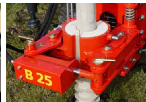
Hydraulic clamp for guiding the screw foundations
