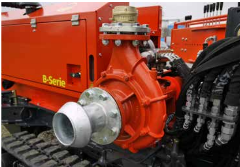
Powerful water pump 120 m³ / h at 8 bar – extendable for maintenance
