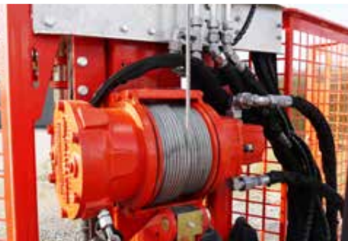
Winch with 5 kN (500 kg) tractive force
