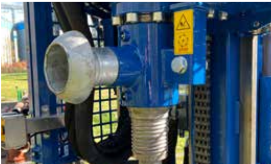
Head preventer with side outlet
