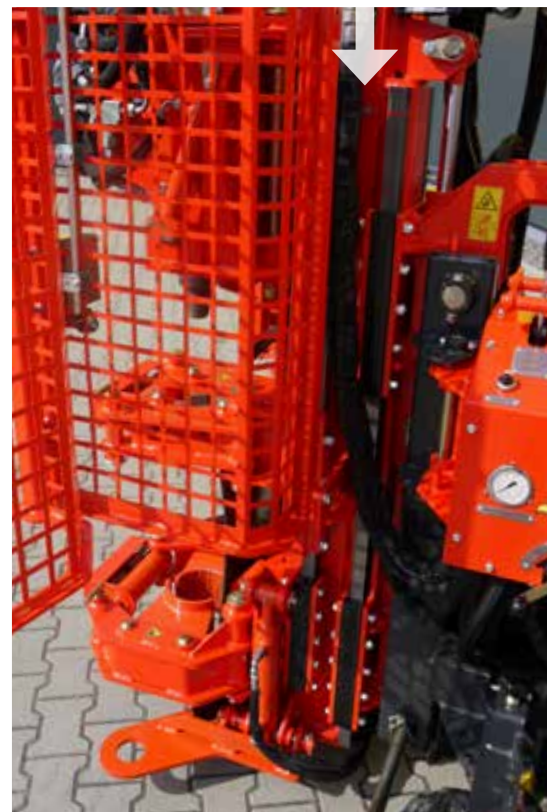
Hydraulic mast lowering 300 mm on the B 50 and B 75
