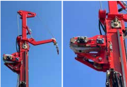
Mast crown with rope sling
