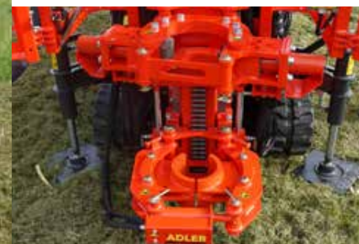
Cable-crushing-lifting clamp up to 11.8 tons retraction force
