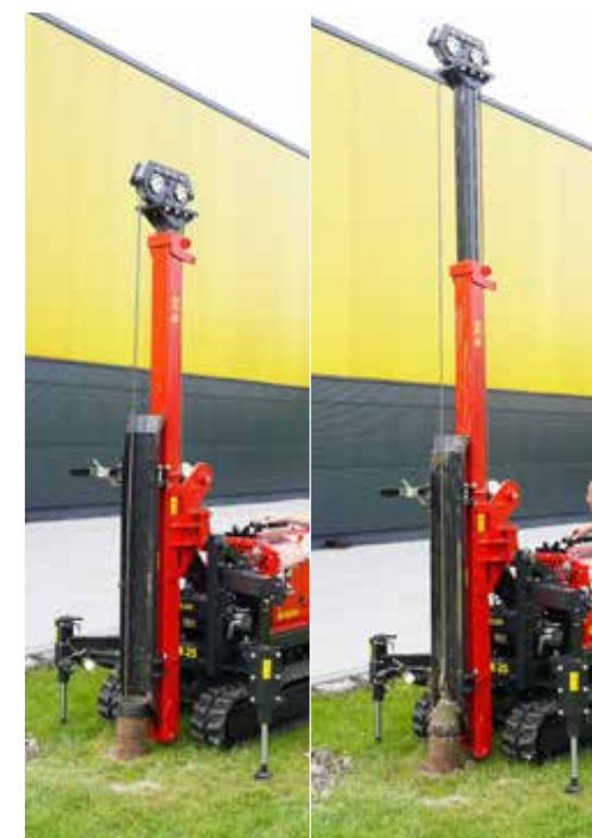
Hydraulic mast extension 1,000 mm
