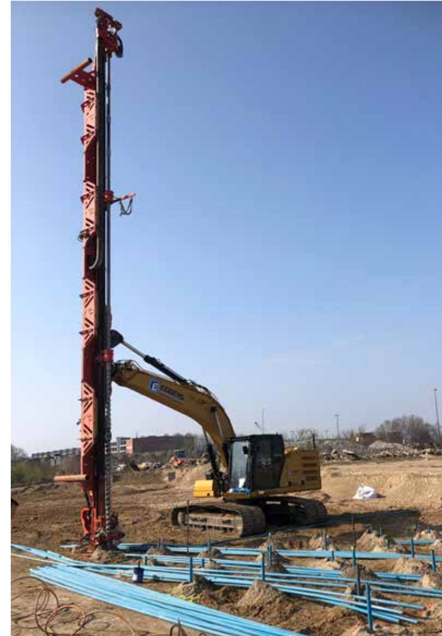
ADLER-ABL 12 for the probing for unexploded bombs
