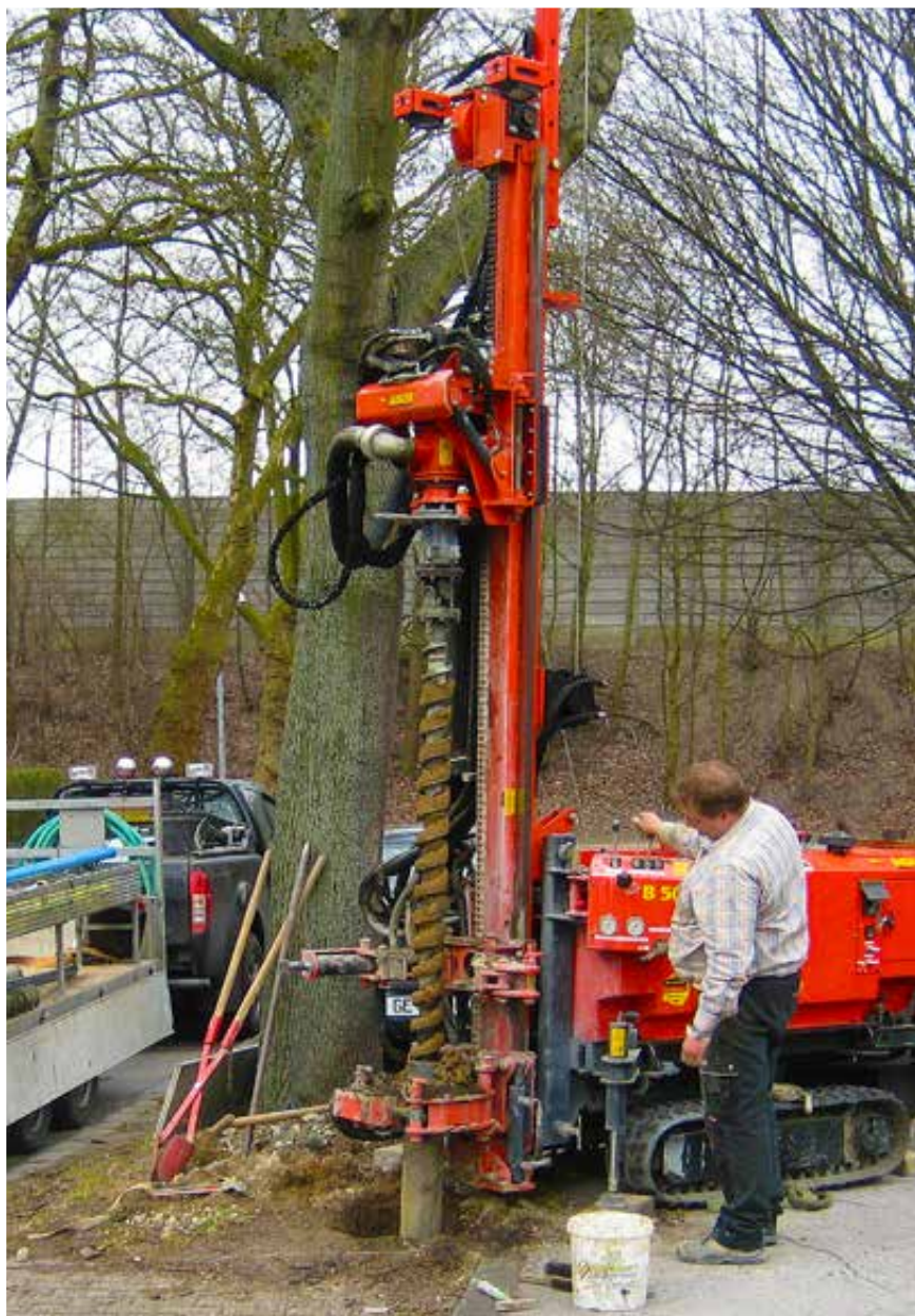
Due to its compact design, the B50 with dry drilling equipment is also suitable for use in confined spaces
