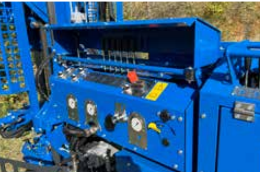
Protective bonnet for operator's platform with illumination
