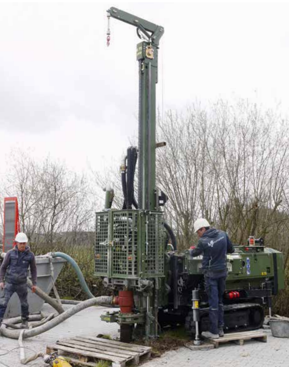
Flush drilling with water circuit via a container
