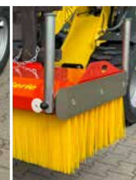
Swivel-mounted parking supports in the parking and working positions
