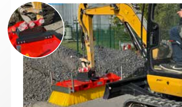
... and fitted with a quick-change system on the excavator
