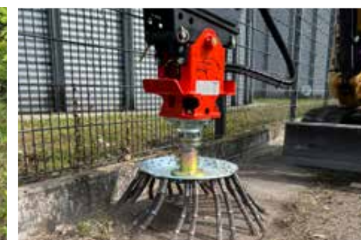
Increase in area output by swiveling the excavator
