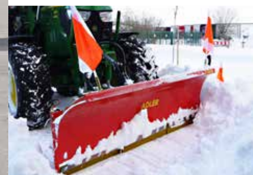
Snow blade, material thickness 5-6 mm steel plate
