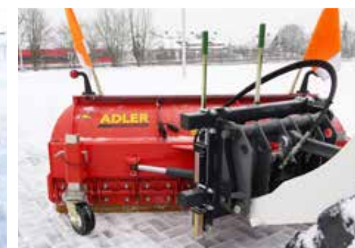
Heavy universal mount system with hydraulic pivot mechanism (with two hydraulic cylinders)
