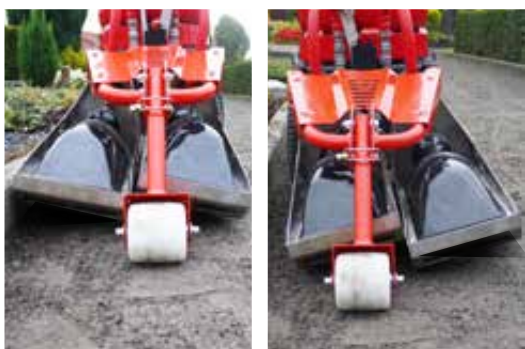
By tilting the emitter to the right or left, even edges can be easily treated
