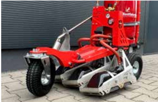
With large steerable support wheel for difficult terrain
