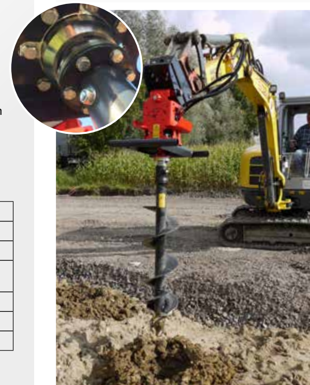
Universal joint and support bearing as standard
