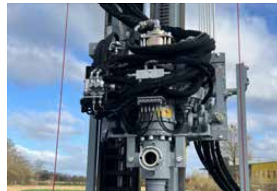
Drill head in the drilling center
