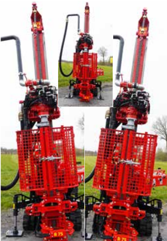
3D mast tilt by 5° (forward and side) as standard
