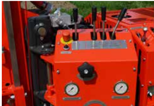
Control panel for controlling the drill head
