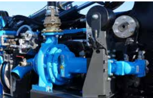
Powerful water pump with up to 120 m³/h or max. 12 bar
