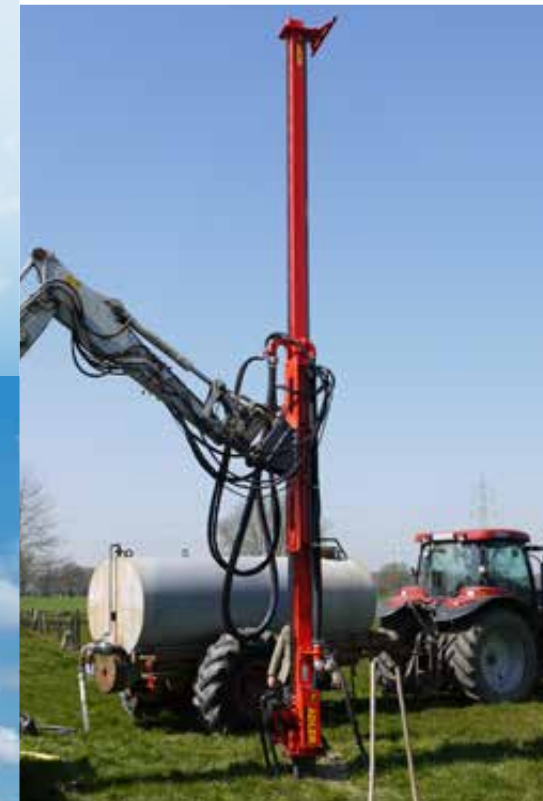
Attachment drill mast with 6.5 m travel on the 8 t excavator
