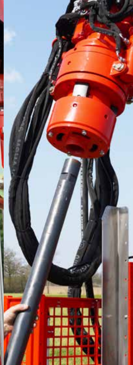
Hydraulic clamping bell (large/small) for breaking the drill pipes and the outer pipework up to 178 mm (only possible with large clamping bell)
