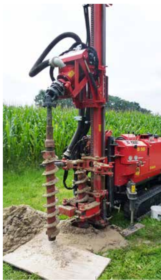
Easy disassembly of the hollow stem auger due to the swivel-out drill head
