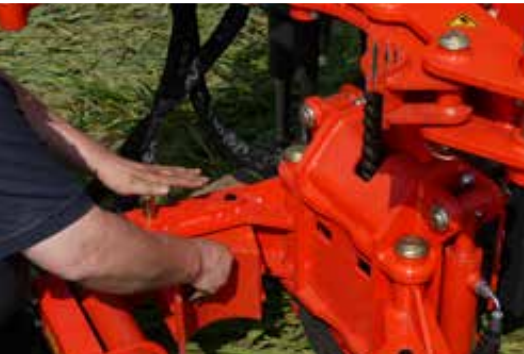
Lifting clamp with exchangeable jaws
