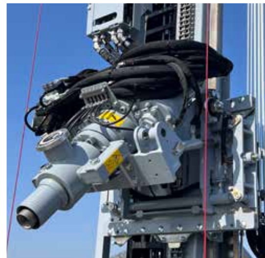
Forward-tilting drill head with integrated head preventer
