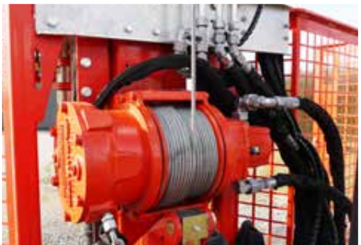
Winch with 5 kN (500 kg) tractive force
