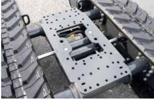
The center piece of the undercarriage has many fixing points for customer-specific use
