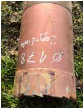
Pipe cutting shoe for Outside piping Ø from - mm to 324 mm
