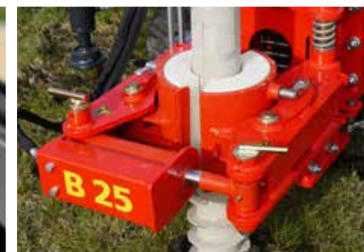
Hydraulic clamp for guiding the screw foundations
