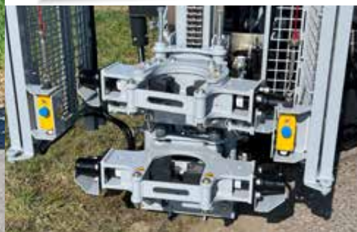
Clamp-break lifting clamp and lower clamp
