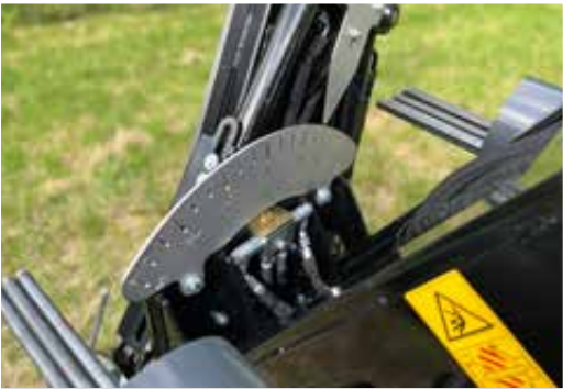
Angular measuring unit for oblique hammering
