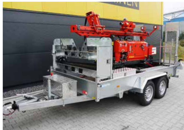
Drill transport trailer dead weight 560 kg and gross vehicle weight 3,500 kg, incl. loading ramp
