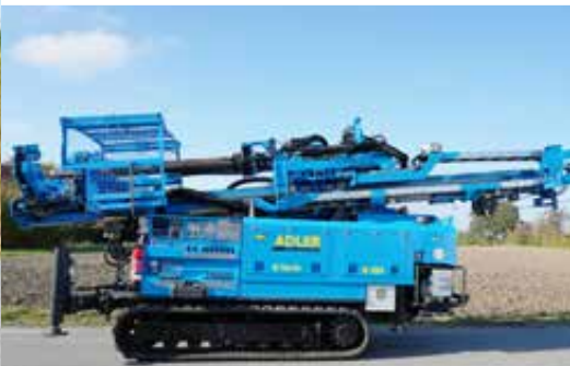
B 200 with folded drill mast in loading position for transportation to the construction site
