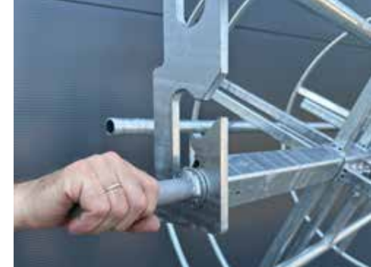
Easy hooking of the reel into the lifting frame
