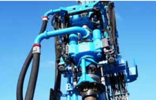
Double-head drilling drive with clamping bell for simultaneous sinking of the drill pipe and outer casing for overburden drilling
