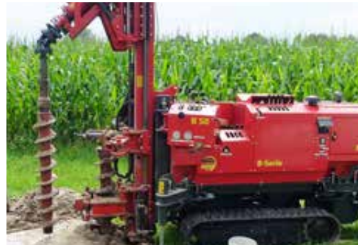
Drilling with hollow stem auger and universal joint
