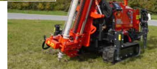
15° mast tilt to the right / left / front
