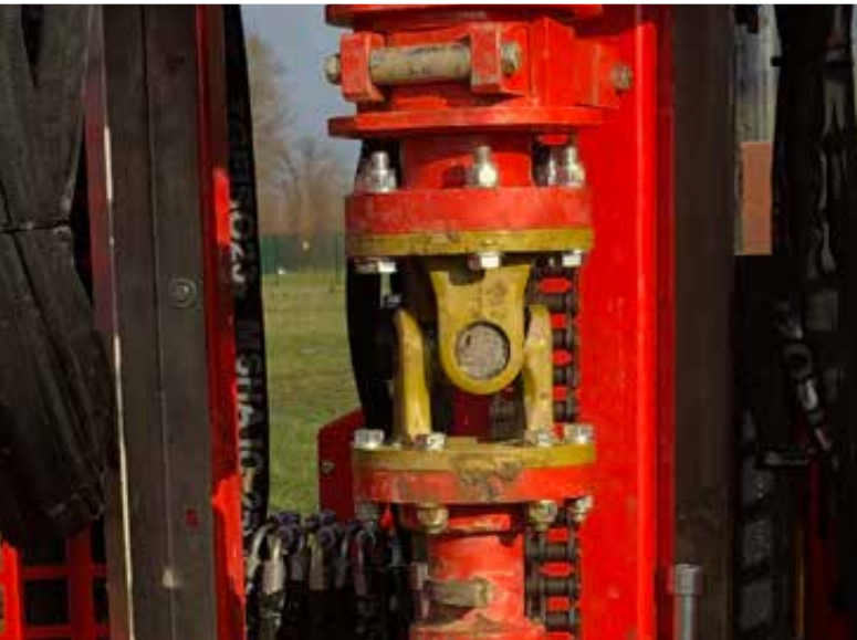
Universal joint with BOM 73.5 above, SW 41/51 below
