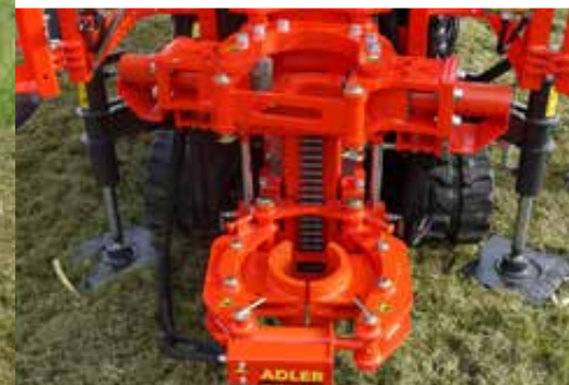
Cable-crushing-lifting clamp up to 11.8 tons retraction force
