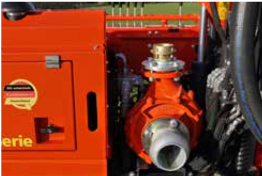
Mud pump "on board"
