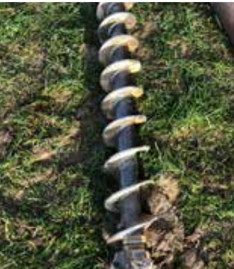
Drill starter with endless screw of 80 mm available up to 324 mm
