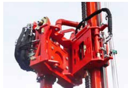
Hydraulic pivoting of the drill head from the drill centre
