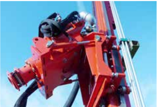
2-stage drill drive with torques up to 620 daNm or revolutions up to 210 rpm
