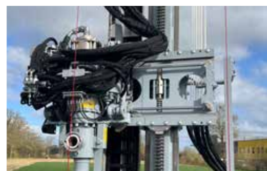
Drill head hydraulically displaced from the drilling center
