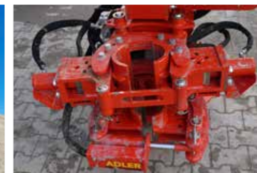
Mast foot designed as a cable-crushing-lifting clamp
