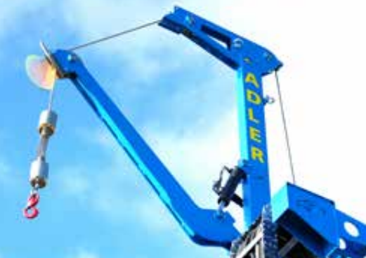
Hydraulic mast extension with a hook load of 17.5 kN for convenient feeding of the drilling tool
