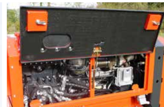
Drill rig B 75 equipped with 75 HP and 2.9 litre Deutz engine of the latest emission standard 5
