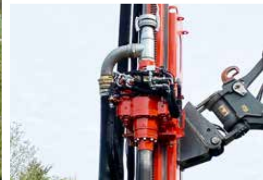
Attachment drill mast with hydraulic clamp
