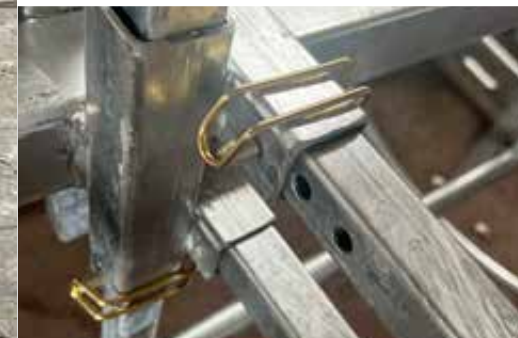
Adjustable inner diameter using locking pins to match the specific probe
