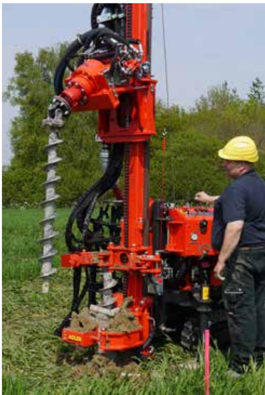
The auger is removed by swivelling out the drill head
