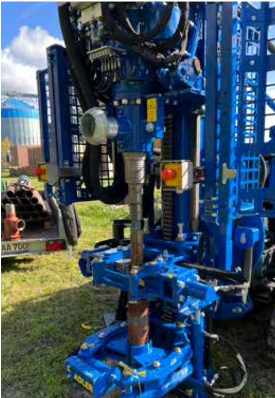
Cable-crushing-lifting clamp in use
