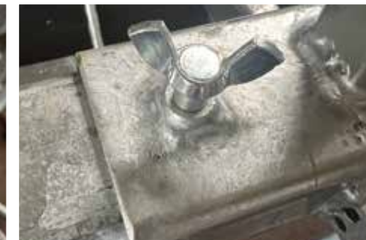
Tool-free adjustment of the reel wheels to suit the respective probe package
