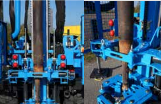
Clamp break lifting clamp for easy breaking of the drill pipe and outer casing with casing clamp at the bottom
