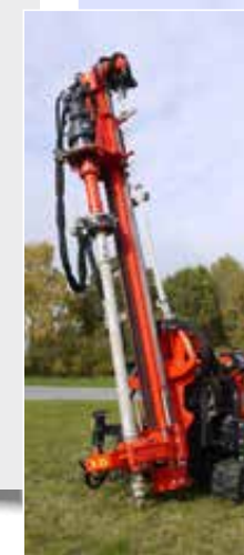
Variable drill head with up to 8,000 Nm and with quick change device
