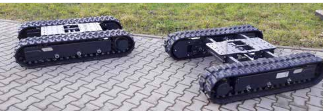
The undercarriages can be manufactured either hydraulically telescopable or without a center section
