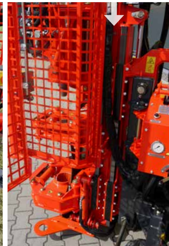
Hydraulic mast lowering 300 mm on the B 50 and B 75
