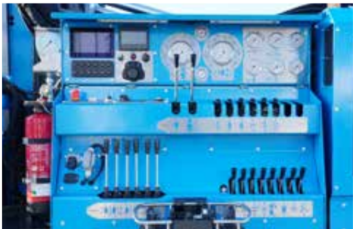
Control panel with all instruments and displays for monitoring the drilling process and the drive unit (Deutz engine)
