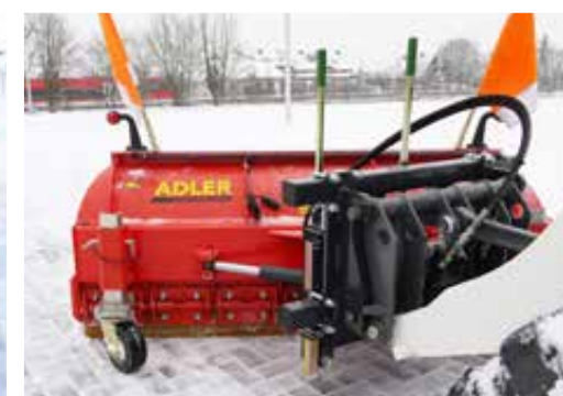
Universal mount system with hydraulic pivot mechanism (with two hydraulic cylinders)
