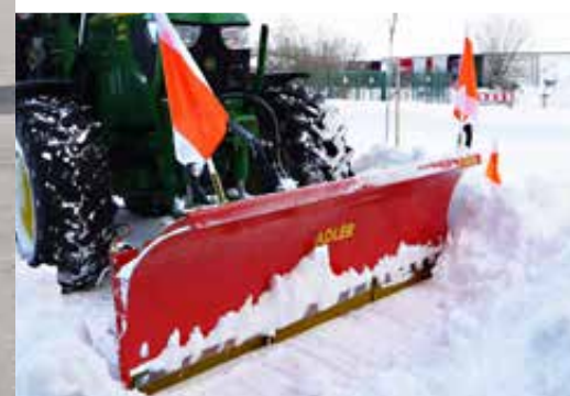
Snow blade, material thickness 5-6 mm steel plate
