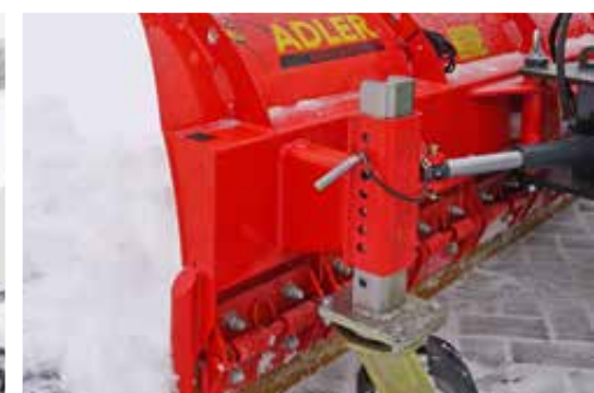
Height-adjustable support wheels (200 x 80 mm)
