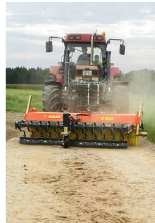
KV-series Scraper Attachment with third support wheel
