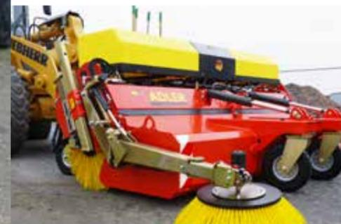
Optional hydraulic side brush, can be switched on/off (ø 900 mm).
