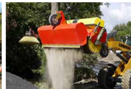
Hydraulic hopper emptying system
