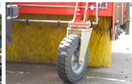
Three large wheels 400 mm x 100 mm
