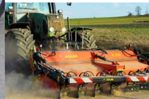
K 750 with hopper and Scraper Attachment
