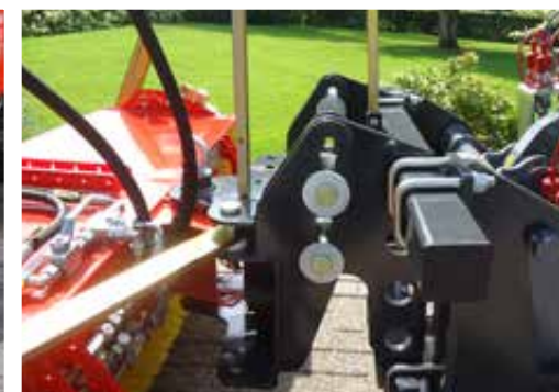
Yard loader attachment with 3D levelling system
