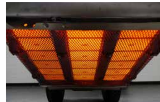
Infrared radiation without naked flame
